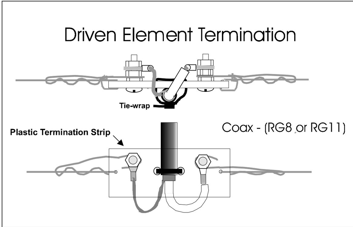
Note: These terminals are not supplied when Cubex Matching Transformer is ordered with Antenna
