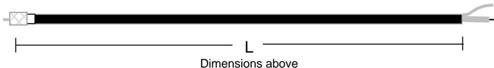
**For 3/4 wave lengths multiply the lengths above by a factor of 3, excess cable may be coiled into a 6 inch dia. Coil and taped together.**
