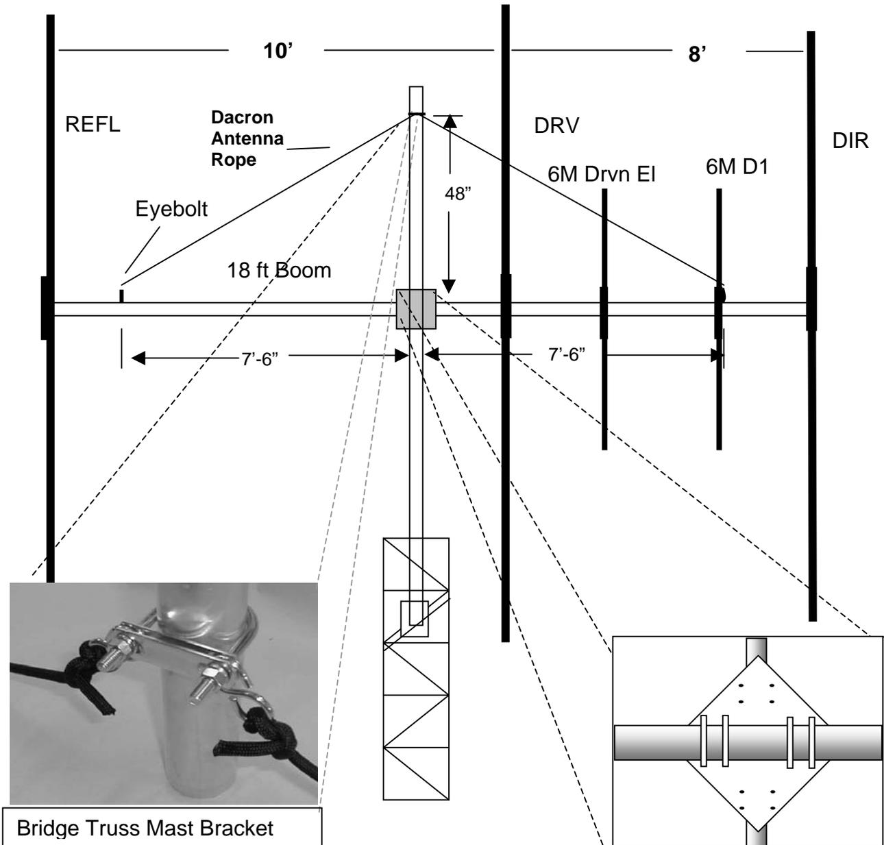
In the SKYM III and SKYM IV antenna models an appropriate length of high quality UV resistant Dacron antenna rope is supplied along with necessary eyebolts to complete the truss guying of the boom. Eyebolts for a 2" mast and 3" boom are supplied and the boom holes are pre-drill for proper location of the truss line.
