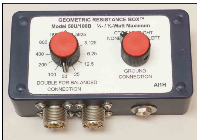
Fig 10—The AI1H geometric resistance box. It is designed to provide both unbalanced and balanced resistive loads.
