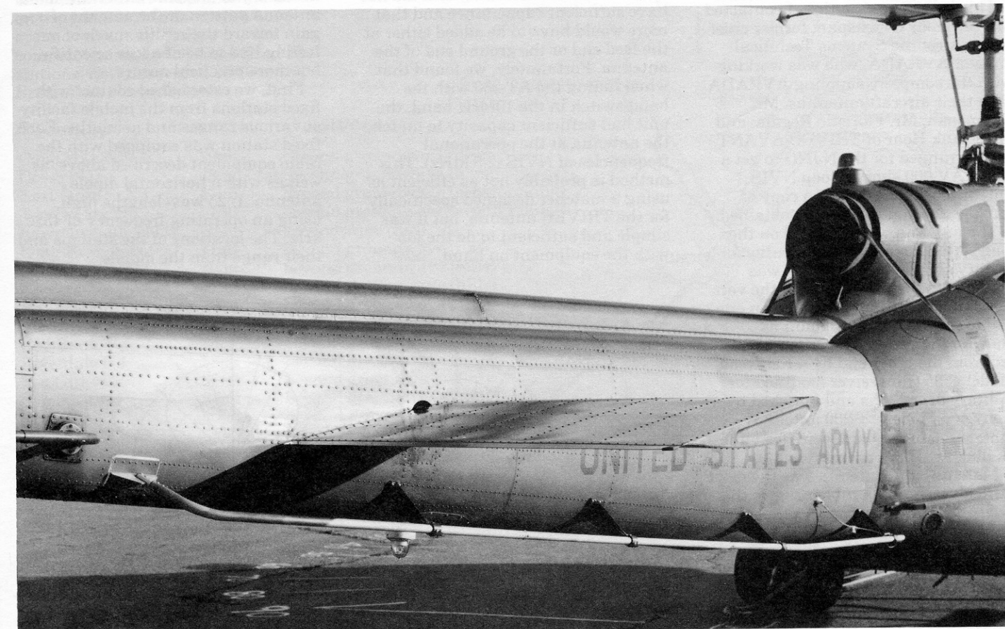
Figure 2. Series AV-600 NVIS antenna installed on Army UH-1
